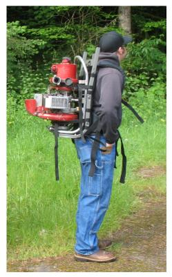
The Mark 3 pump is commonly in the line-up of firefighting equipment used throughout the western states. While the Mark 3 has plenty of horsepower and can move lots of water, it weighs in at 55 pounds, making it awkward to pack very far from the truck... and a back injury just waiting to happen.
